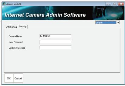
You can change IP camera's name, and change its administrator password here by inputting new password in both 'New Password' and 'Confirm Password' field.
